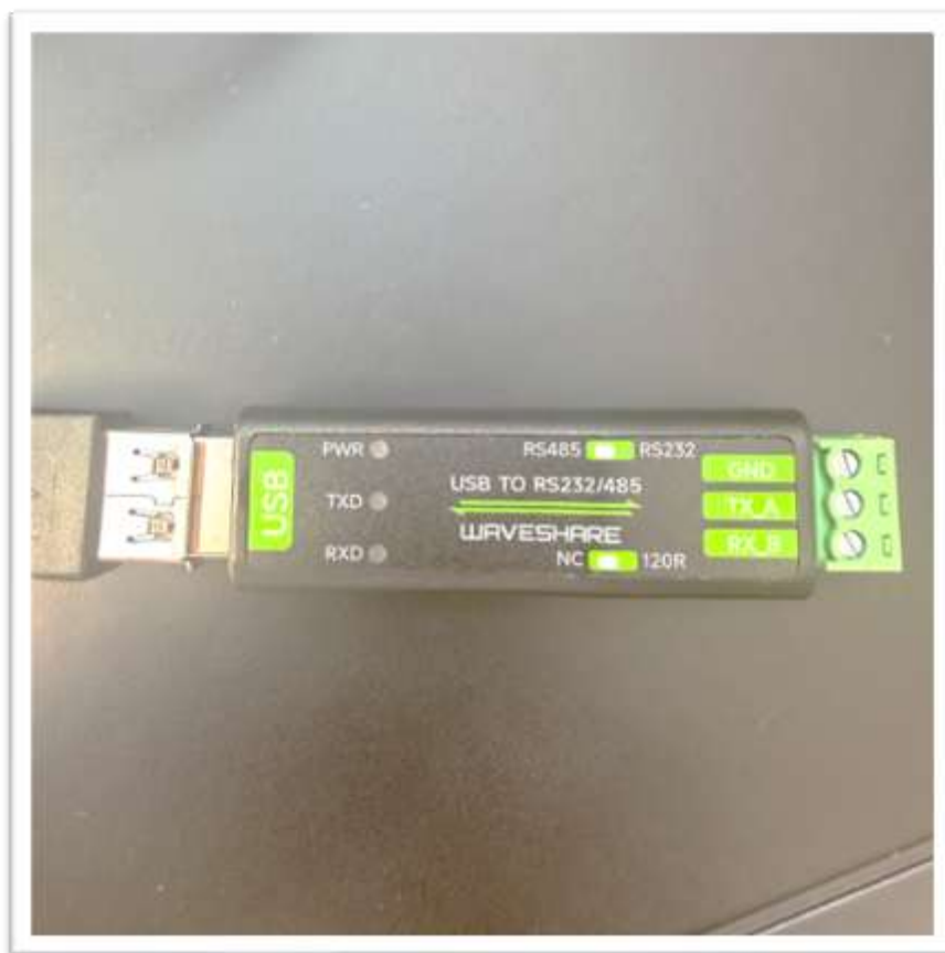
USB-to-RS-232 commissioning adapter example. Select RS-232 mode.
